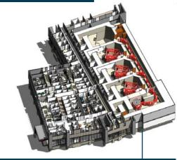
The layout of the equipment with the beam being taken from the cyclotron (particle accelerator) to the three treatment rooms. The fourth room funded by The Christie charity will be used for research.
